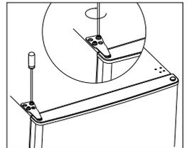
12. Put the hinge cover and the screw cover back.
