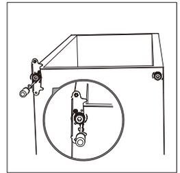
11. Place the door back on. Ensure the door is aligned horizontally and vertically so that the seals are closed on all sides before finally tightening the top hinge. Insert the hinge bracket and screw it to the top of the unit. Use a spanner to tighten it if necessary.
